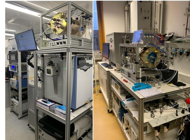
Fig. 2: a) Orbitrap-MS system inside the ALFA measurement container; b) Orbitrap-MS setup for laboratory experiments
